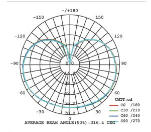
All luminous intensity values (shown radially from centre are in cd. Elevation angle values are shown around the outside of the graph.
