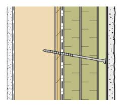
Screw at Upward Angle (Section View)
