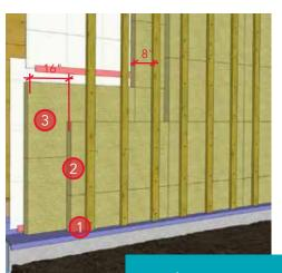
An alternative installation approach is to use one or two fasteners with washers to pin the insulation boards in place before the strapping is installed.
